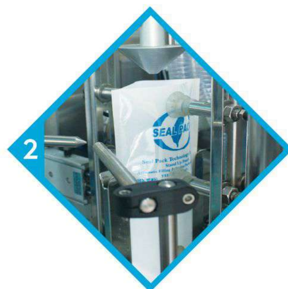
◆ 2 Automatic Opening Station
